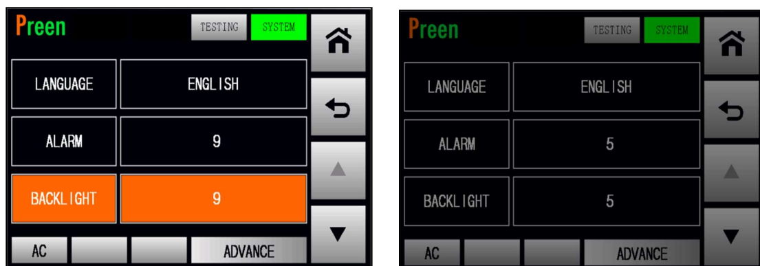
Figure 3.37 Set the backlight level from 9 to 5
