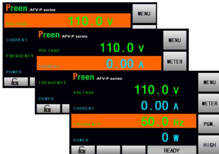
Figure 3.3 Move the cursor on the touch screen by turning the rotary knob
