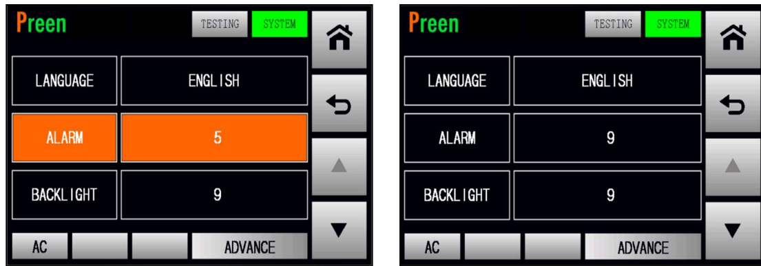
Figure 3.36 Set the alarm volume from 5 to 9
