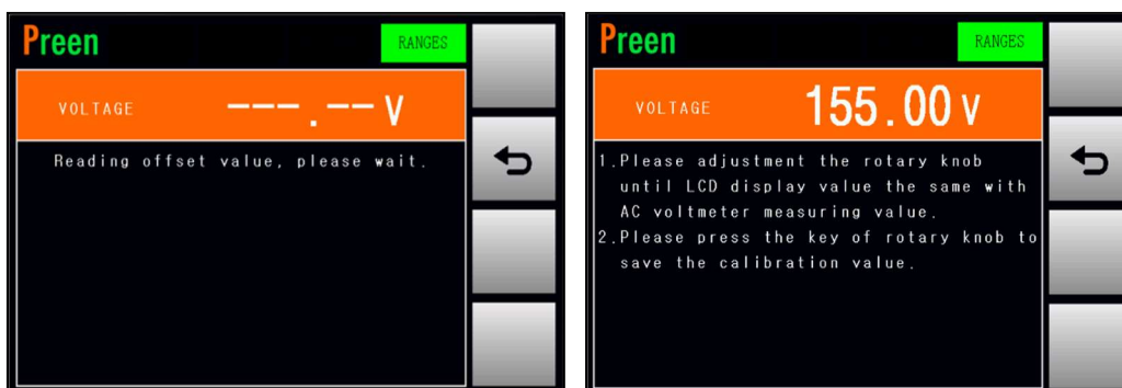
Figure 4.8 Enable the calibration of the LO-Range voltage 155V
