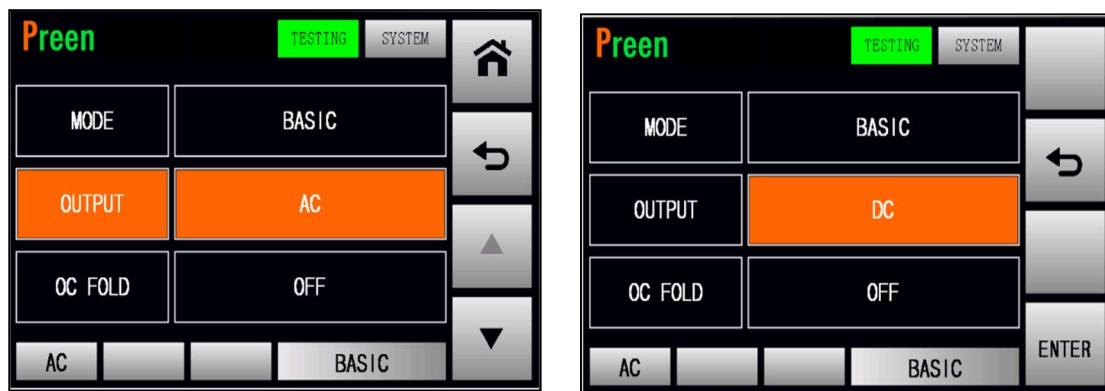
Figure 3.26 Set the output mode from AC to DC (BASIC mode)
