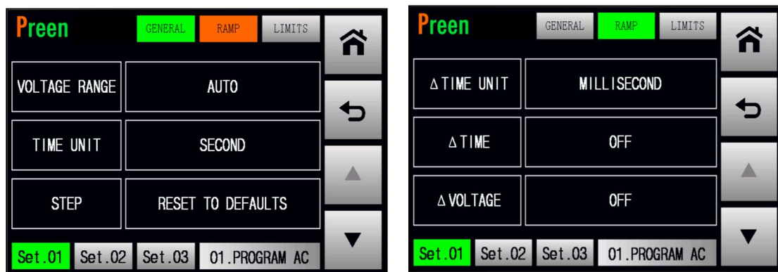
Figure 5.13 Enter into the RAMP subpage
