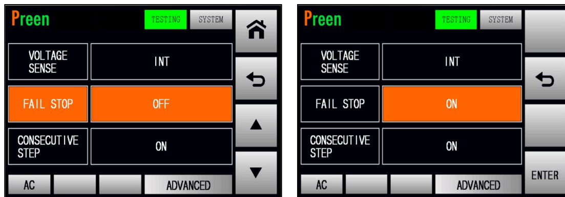
Figure 3.21 Enable the fail stop feature (ADVANCED mode)
