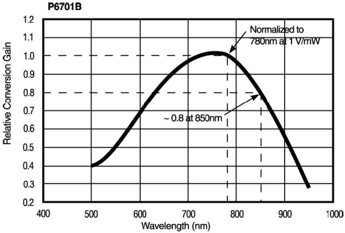
**Figure 3: P6701B typical wavelength dependent gain (25 °C)**
