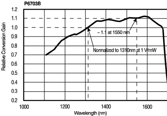
**Figure 4: P6703B typical wavelength dependent gain (25 °C)**
