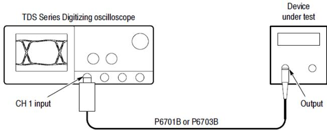
**Figure 5: Setups with the TekProbe II interface**
